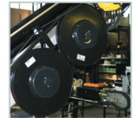
Activations powered by means of hose winder Activaciones alimentadas con arrolladores de tubos
