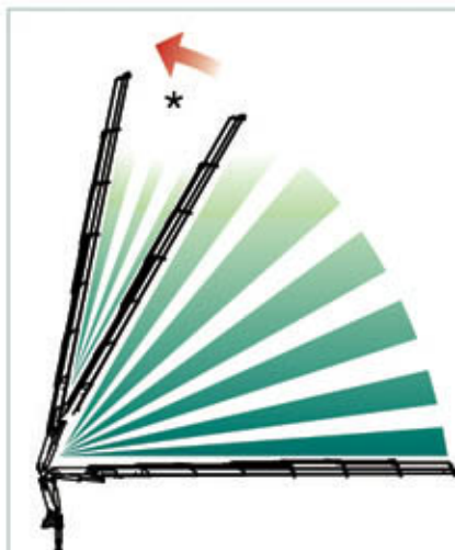
* Area controllata elettronicamente - Electronically -controlled area
