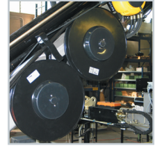
Activations powered by means of hose winder. Activaciones alimentadas con enrolladores de tubos.
