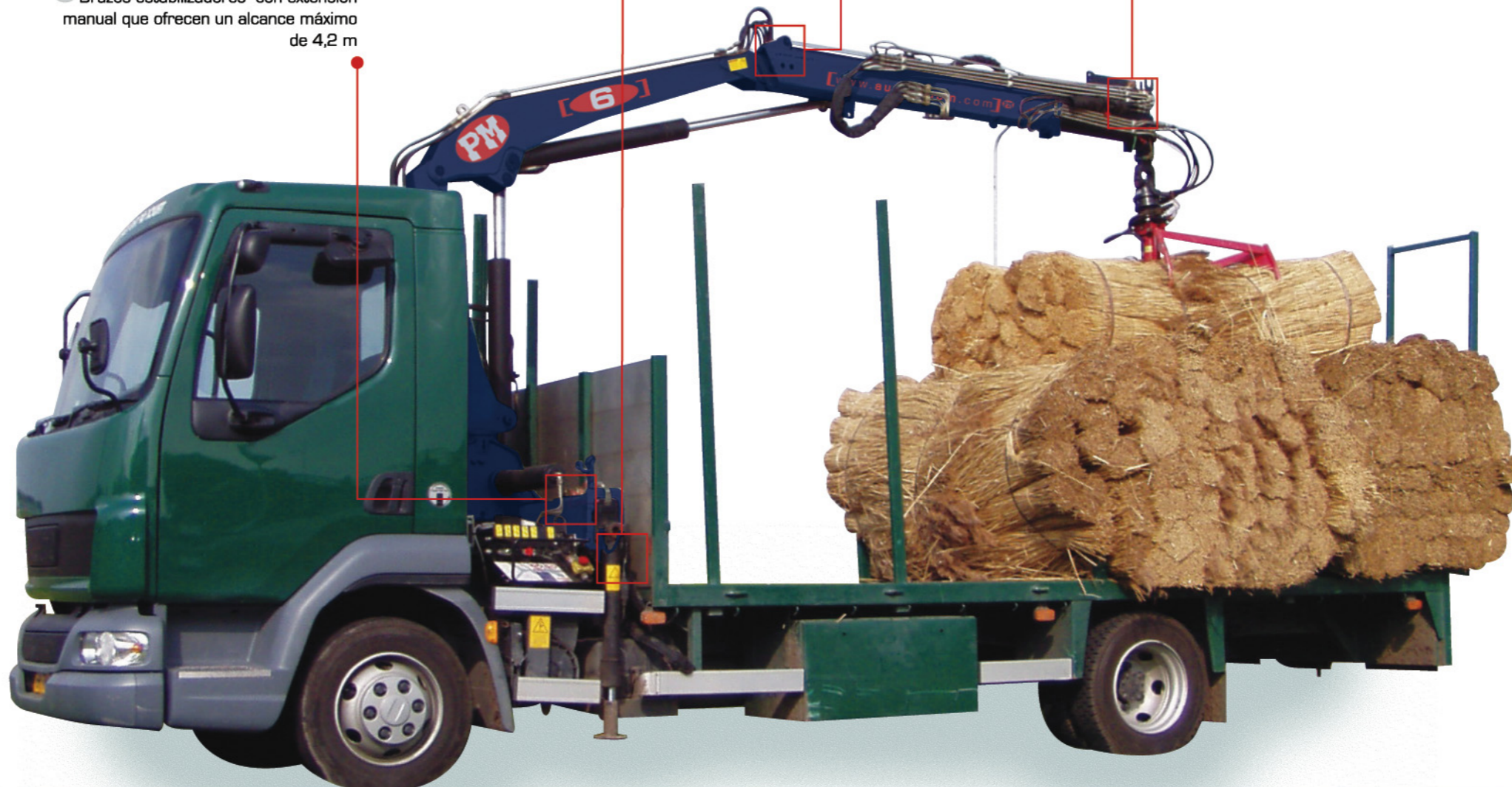
Hydraulic winches with a capacity ranging from 2090 lbs up to 2430 lbs on cranes. Cabrestantes hidráulicos de 950 kg a 1100 kg en grúa.
