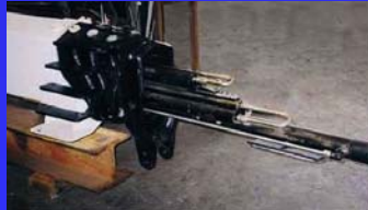
Internal cylinders offer improved protection. All cylinders can be removed simply by taking off the hinge pins.
