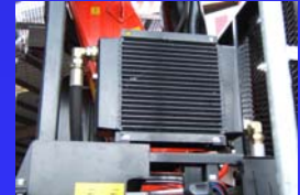
Hydraulic oil cooler for constant temperature of oil in extreme conditions.
